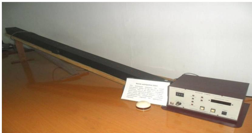
This apparatus measures the visual anticipation ability of the player in static condition. This is an index perceptual motor skill required in anticipation of time – lapse before the onset of stimulus and the perceptual – motor conditioning (eye-hand coordination) required for appropriate reaction.
