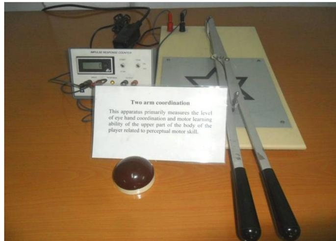
This apparatus primarily measures the level of eye-hand coordination and motor learning ability of the upper part of the body of the players related perceptual motor skill.
