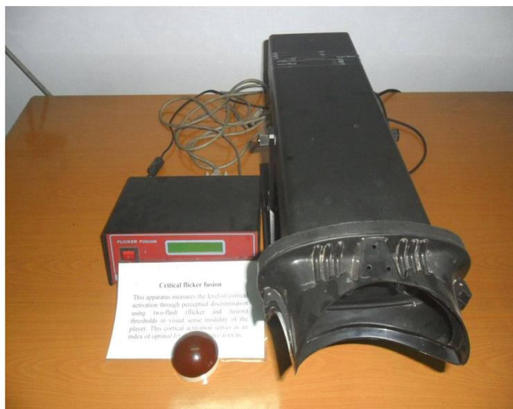
This apparatus measures the level of cortical activation through perceptual discrimination using two-flash (flicker and fusion) thresholds in visual sense modality of the players. This cortical activation serves as an index of optimal level of cognitive activity.
