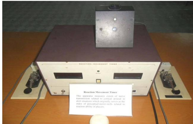
This apparatus measures extent of nerve transmission related to cortical arousal in alert situations which originally serves as the index of perceptual motor-skills related to reaction ability of players.
